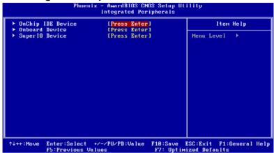
**NOTE:** This "Integrated Peripherals" option controls the configuration of the board's chipset, includes IDE, ATA, SATA, USB, AC97, MC97 and Super IO and Sensor devices, this page is developed by Chipset independent.
